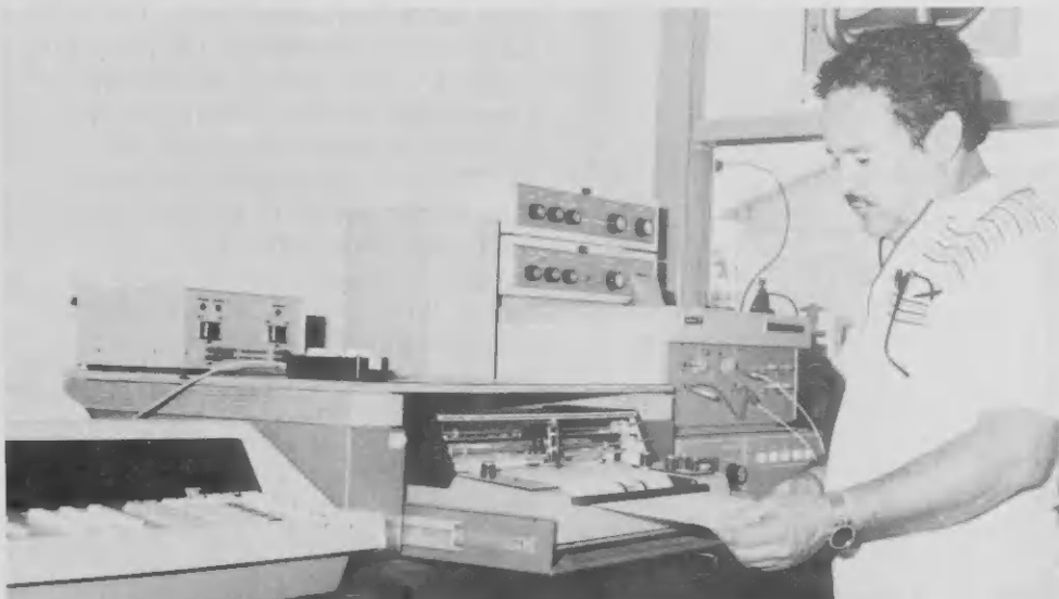
Wing Vrolijk runs a Gas Chromatograph analysis of butane prior to approval for export.
